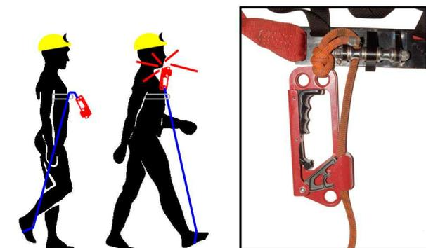
**Figs. 5 & 5A:** Warning! Tension on the foot line while walking will cause the ascender to pivot abruptly upward and it may strike you in the face! Clipping the ascender into the foot line (right photo) will prevent this.
